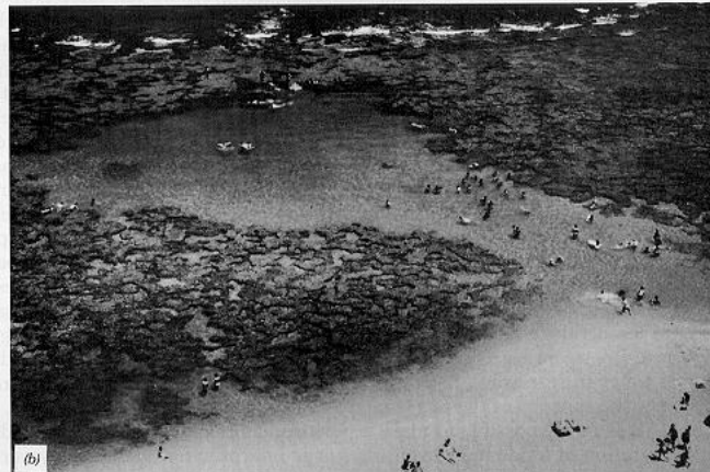
Figure 4.20 Black and white copies of color and color infrared photographs, Hanauma Bay, Island of Oahu, Hawaii: (a) normal color film (0.40 to 0.70 \mu\text{m} ); (b) color infrared film with a Wratten No. 15 filter (0.50 to 0.90 \mu\text{m} ); (c) color infrared film with a Wratten No. 29 filter (0.60 to 0.90 \mu\text{m} ); (d) color infrared film with a Wratten No. 87 filter (0.74 to 0.90 \mu\text{m} ).
