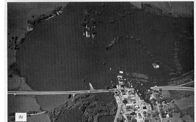
Figure 4.24 Black and white copies of panchromatic and color infrared aerial photographs showing flooding and its aftereffects, Pecatonica River near Gratiot, WI: (a) USDA-ASCS panchromatic photograph. Scale 1:9000. (b) Oblique color infrared photograph, June 30. (c) Oblique color infrared photograph, July 22. (d) Oblique color infrared photograph, August 11. The flying height for photos (b) to (d) was 1100 m.
